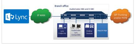
Branch office users can benefit from high definition voice quality with AudioCodes' Lync-compatible IP Phones. Legacy analog equipment such as fax machines can continue to be used in the Lync environment via AudioCodes' field-proven analog gateways. Additional enterprise communications software solutions (such as SmartTAP Call Recording, Fax Server and Auto-attendant) are available as optional add-ons to the existing branch gateway or E-SBC platforms.
