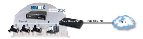
(Note: The SNBX, or SmartNode Branch eXchange, in the application image is a Patton appliance used to run 3CX Phone System.)
